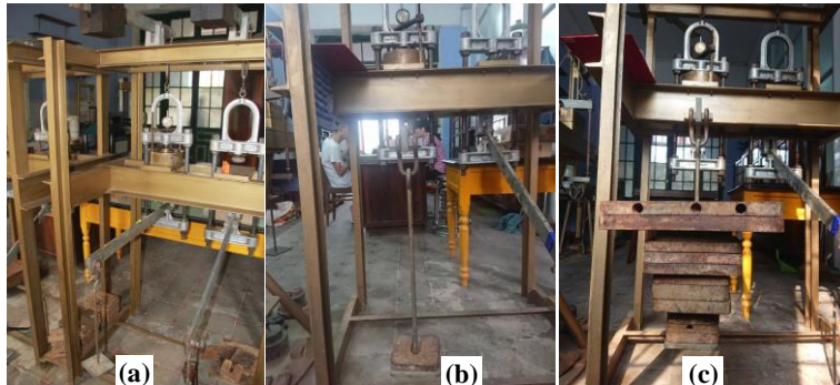
Fig. 2. Standard one-dimensional consolidation test at different stages: (a) Test box including soil specimen before loading, (b) first load increment and (c) final load increment
